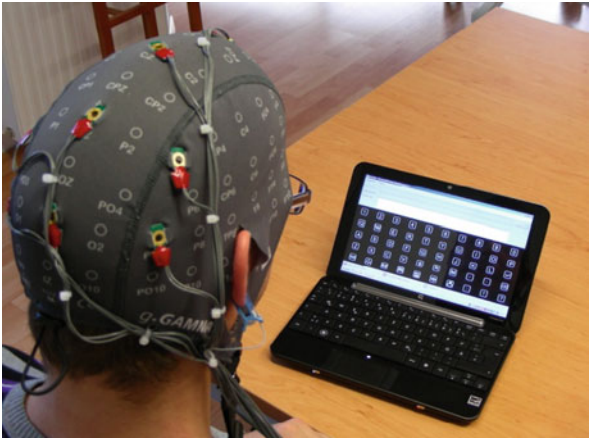
Fig. 14 Intendix running on the laptop and user wearing the active electrodes
