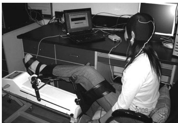
Fig. 9 A system used for lower limb rehabilitation. The motor imagery based BCI is used to control the device. Positive rehabilitation training is performed in accordance with the concurrent motor imagery of foot movement
